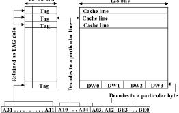
Figure 3: Physical Address Mapping
