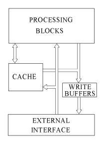
currently stored in the cache. If the data is cacheable and is not currently in the cache, the data is written out to system memory. On the Blue Lightning SX2 and SX3 a line fill request for that physical address is then made. This approach, known as write-allocate, causes the system memory to be updated first and then that line to be read into the cache.
