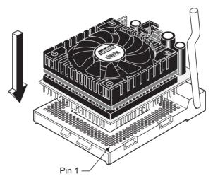
Figure 5: Orienting the TurboChip
