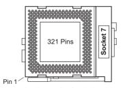
Figure 3: Empty Socket 7 Top View
