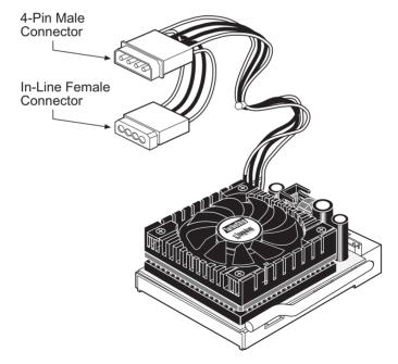
Figure 7: Attaching the Power Cable
