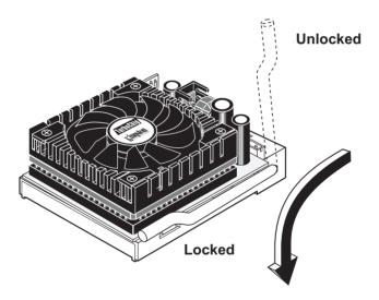
Figure 6: Securing the ZIF Socket
