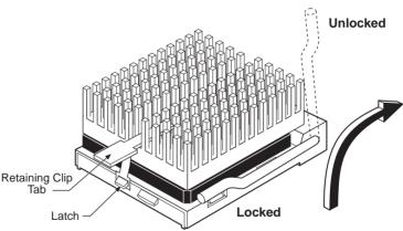
Figure 4: Removing the CPU Chip
