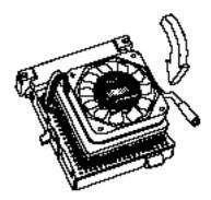
Fig. 2-7 Securing the ZIF Socket
