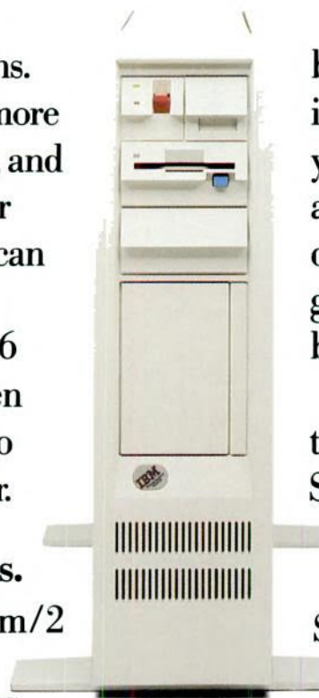
The IBM Personal System/2 Model 80 was created to unleash the power of the 80386 microprocessor.
